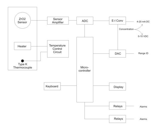
Figure 2-3: Signal Processing Block Diagram
